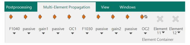
It uses two separated filters at 1030 nm and 1040 nm as well as passive and active fibers in between. The gain fibers are different after the filter. An output coupler is used at the end.
